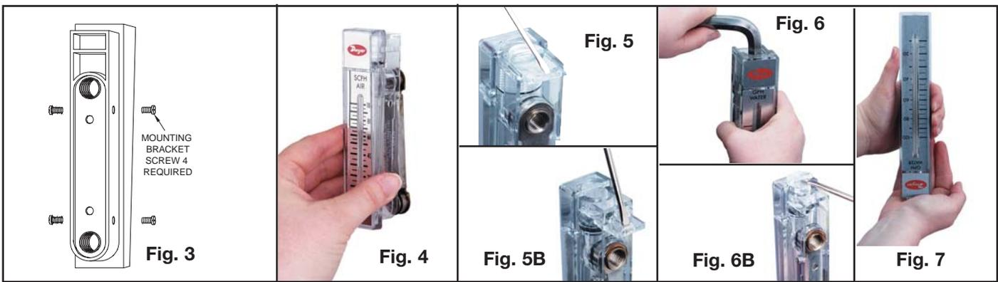
**Surface Mounting:** Drill appropriate holes in panel, using the dimensions shown in Fig. 2. Hold the flowmeter in position in front of the panel and install the clamp bolts from the rear. (The mounting clamps may be used as washers, if desired, by installing them backwards or straightening them out.) Pipe up inlet and discharge following the directions in the previous sections.
